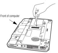
(Sample Illustration) Unscrewing the memory module slot cover
